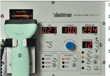
Tine adjastment for timer and current After setting the function you can adjust the timer and the current level can be adjusted to suit your needs.
